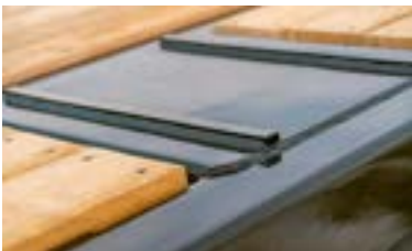
Heavy duty grosser bars on wheel covers for improved traction
