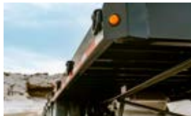
Formed 8" side rail constructed from 100,000 psi hi-tensile steel
