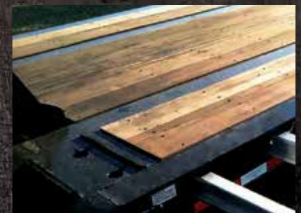
Apitong hardwood decking resists moisture
